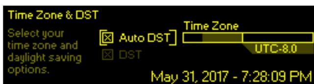
The screenshot shows the 'Time Zone & DST' configuration screen. The title is 'Time Zone & DST' and the subtitle is 'Select your time zone and daylight saving options.'. There are two checkboxes: 'Auto DST' and 'DST', both of which are checked. The 'Time Zone' dropdown menu is set to 'UTC-8.0'. The date and time at the bottom of the screen are 'May 31, 2017 - 7:28:09 PM'.
