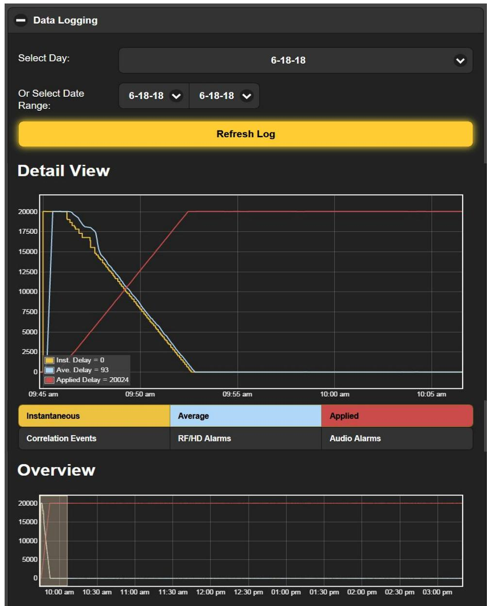
Data logs are accumulated on a 24-hour, daily basis. The log may be called-up with the View / Refresh Log bar to show either the current day to the current time, as in this example, or to show an entire previous day, or even to display a number of sequential previous days as specified in the Or Select Date Range: fields. The day starts at midnight (or whenever the JUSTIN 808 is placed in service if less than 24 hours).
