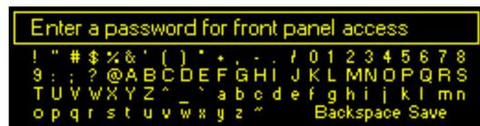
For extended operation from the front-panel, you can navigate to Admin / Display and set Timeout to a temporary period of the maximum, 60 minutes. You may also remove the password by navigating to Admin / Security. The password will be visible, so write it down so that you can re-enter it to restore front-panel security. Use Backspace to remove the password and then select Save.
