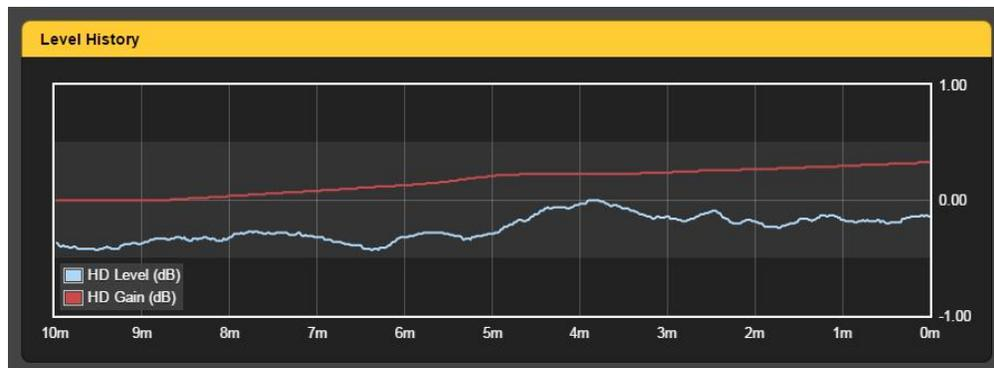
It should be possible to hold the HD level within  $\pm 1$  dB of the FM program channel; the graph Y scale auto-ranges to keep the plots on the screen. Nevertheless, and especially with independent audio processing setups, that blue line is bound to wander a bit.
