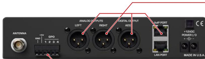
Fulltime off-air program audio is available simultaneously as L/R-analog, AES3-digital and Dante/AES67 AoIP streaming, all with adjustable levels, plus a multi-listener Internet IP stream and front-panel headphone jack.
