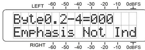
Bytes 1 through 23 (AES 3), or bytes 1 through 5 (S/PDIF), are not decoded to plain text, but are simply shown as a sequence of zeroes and ones. Consult the appropriate Standard for a detailed explanation on what these channel status bits include.
