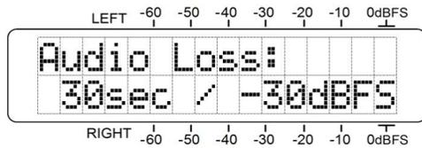
alarm trigger. The delay may be programmed in one-second increments up to 2 minutes. You may also turn the knob completely counterclockwise to OFF to deactivate the alarm altogether.
