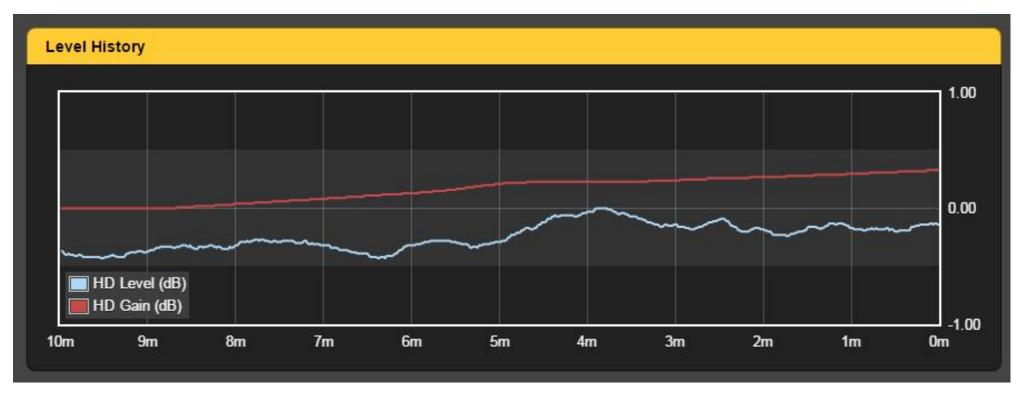
It should be possible to hold the HD level within ±1dB of the FM program channel. But especially with independent audio processing setups, that blue line is bound to wander a bit. The graph scale changes its range to keep the plots on the screen. The JUSTIN 808 data-logging utility does not keep an extended record of this level variance.
