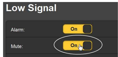
front-panel OLED menu. Turning Mute: On will assure that both the Low Signal and FM Audio Loss alarms will be triggered should the transmitter fail. Otherwise the FM Audio Loss alarm will respond only to 'dead air,' and the Low Signal alarm, alone, will signal a transmitter failure.
