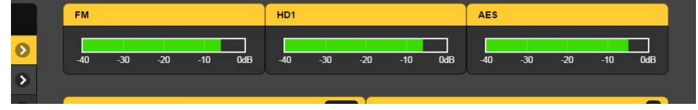
Delay Alignment Metering The front-panel FM-HD1 ALIGNMENT indicator actually performs multiple display functions. If the JUSTIN 808 has not yet achieved correlation between the FM and HD1 programs, a single LED 'hunts' back and forth across the face of this display.
