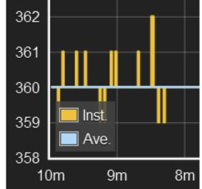
as quickly as the autocorrelation algorithm can calculate them, which with moderate and typical wanderings is pretty darned snappy. The time-averaged Ave. value is the basis for the applied delay, which will eventually bring the measured delay back to zero.
