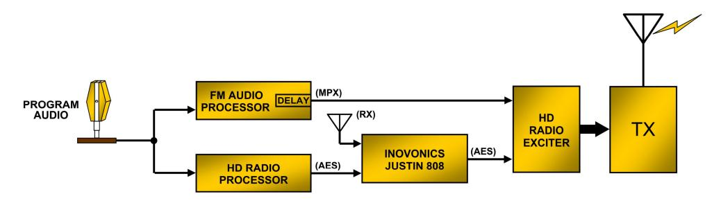
JUSTIN Implementation in HD Radio Air Chain With Dual Audio Processors
