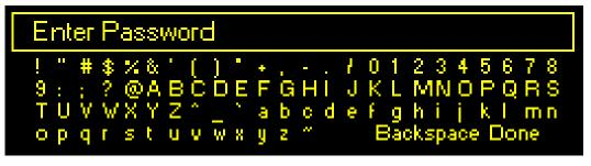
once more. The front panel will become fully accessible until the OLED timeout period has expired, which will then require the password to be entered again.
