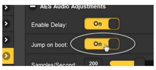
tion, it will correct the delay error and bring the analog FM and digital HD1 programs into time alignment instantly. There really is no valid reason for turning this switch Off, unless the slow alignment recovery following a power glitch is somehow considered a plus.
