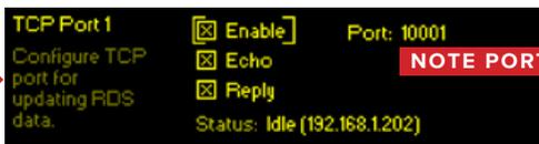
In your automation software, use the IP address and Port number you've noted to "tell" your automation system where to send the data for the Model 732. (This will be different for every automation system.)
