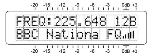
tion. Push the knob and **FREQ** will blink. Turn the knob to tune-in the desired frequency/group.
