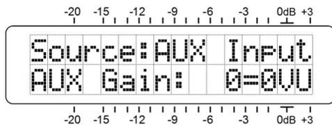
Input sensitivity is normally 'unity': a digital 0dBFS tone will take the front-panel Menu Screen 6 meter to 0dB. You can turn the knob to introduce gain, however, so that the front-panel meter reading of 0dB can equate to 'zero-VU' values of -18dBFS, -20dBFS or -24dBFS.
