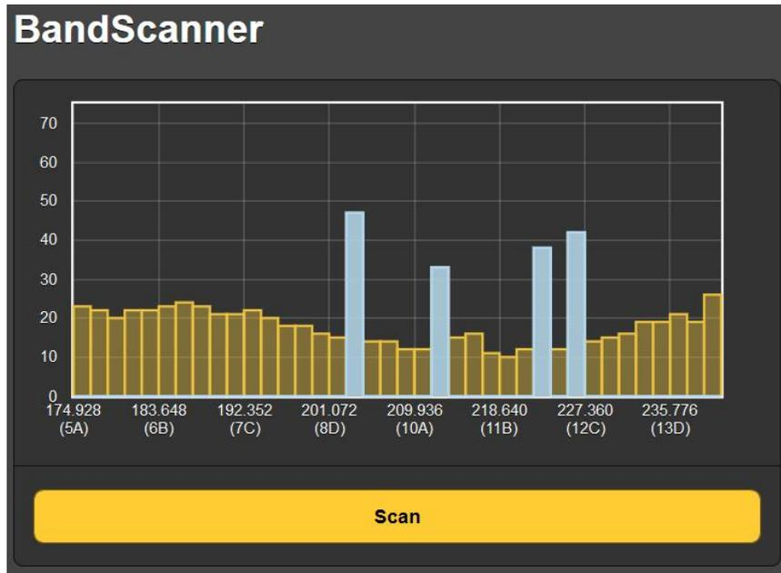
'Hovering' the screen cursor over any DAB carrier (blue bar) will present an information box with the frequency, group, signal level and total number of Services and Components.
