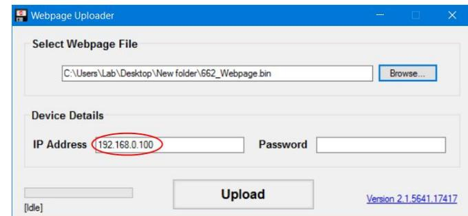
Enter the IP Address, if it does not automatically populate, and then click: Upload. The existing Web interface pages will summarily be replaced with the new ones.
