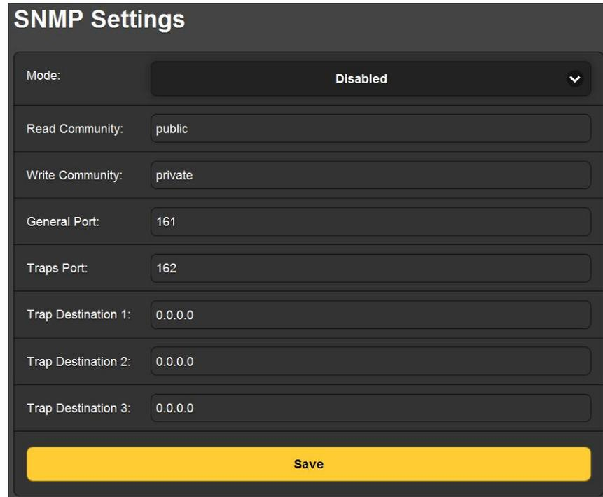
Changing Mode: to Read Only allows the SiteStreamer™ to be interrogated by the SNMP Manager so that SiteStreamer™ settings, metering, PAD data and alarms can be read and integrated by other equipment on the network.
