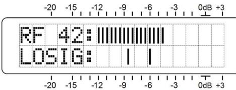
The lower LCD scale is labeled **LOSIG#** and allows local, front-panel adjustment of the carrier loss alarm trigger points.
