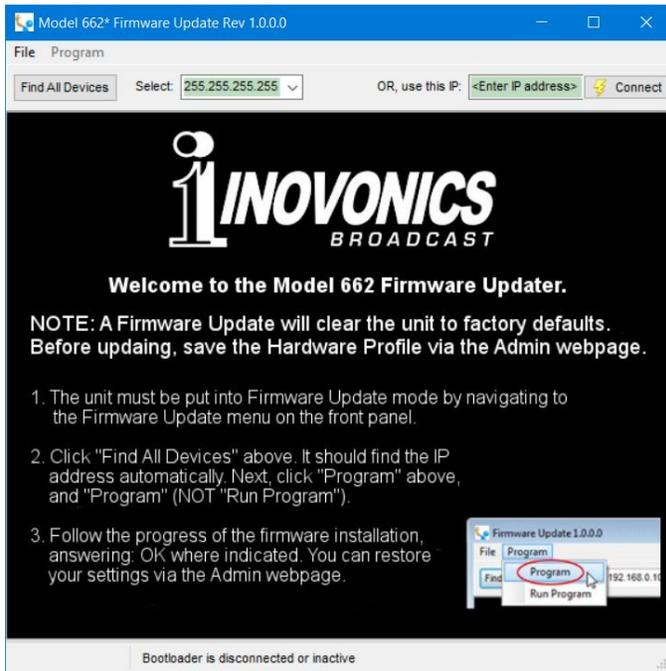
The bootloader window outlines the firmware update process in three easy steps. The first step advises that the SitesStream™ must, itself, be in the 'bootloader' (Firmware Update) mode.
