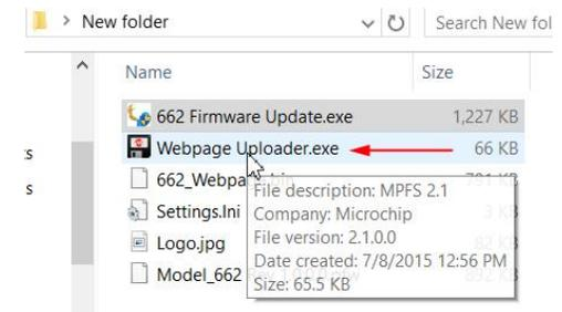
After the firmware update is bootloaded, and while the 662 SitesStream™ is in communication with your computer, return to the New Folder and double-click the Webpage Uploader.exe file to start this utility.
