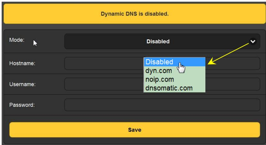
Click on the provider you have chosen, and then type the information into the appropriate boxes on the Dynamic DNS Web interface screen. Follow with a Save. This will allow you to access your SiteStreamer™ when it is behind a dynamic IP address.
