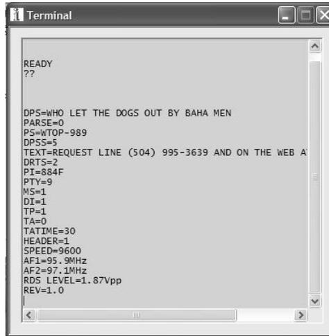
The displayed syntax includes ‘register designation’ headers appropriate to each entry. Any single register may be interrogated by typing its header and a single question mark. For example, type SPEED?↵ to request a confirmation that the encoder port speed is indeed set to 9600 baud.
