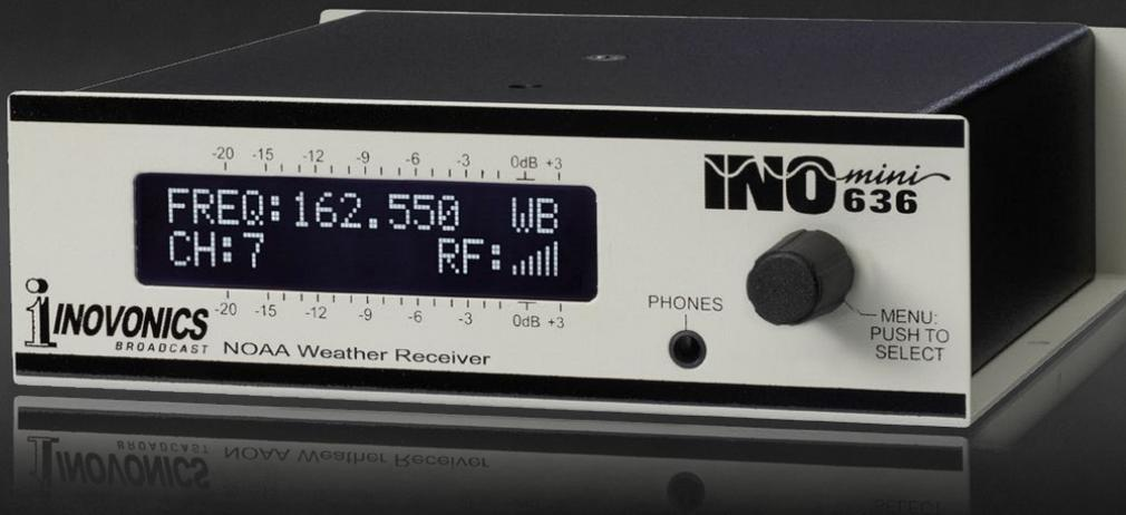
The INOmini 636 is a full-featured NOAA weather receiver in a small-format package. It tunes all weather band frequencies and delivers balanced analog and AES digital audio with automatic intelligibility enhancement for monitoring and rebroadcast. The 636 responds to the 1050Hz Alert Tone and provides alarm outputs for 1050Hz, plus audio and RF loss.
