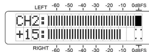
The metering function of this menu displays the peak levels of the digital stereo output signal with regard to 0dBFS. The above illustration suggests that too much gain has been cranked-in, probably driving the signal into frequent clipping.
