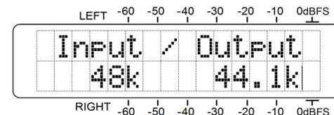
As stated in Product Specifications, the INOmini 300 can lock onto any stable sampling rate between 22.05kHz and 192kHz, even nonstandard in-between rates such as 51kHz.
