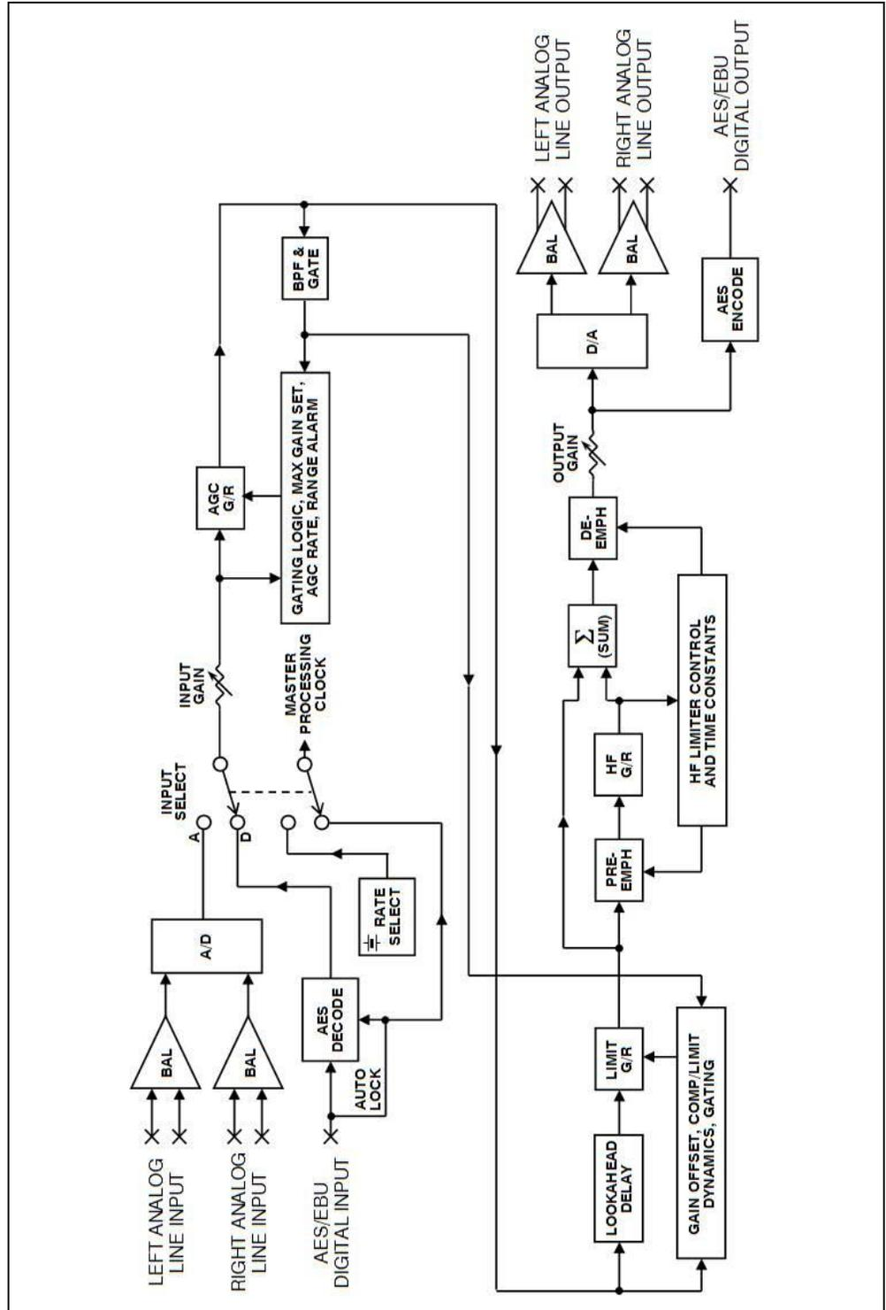
Figure 1 - Block Diagram, Model 261 Digital Utility Processor
