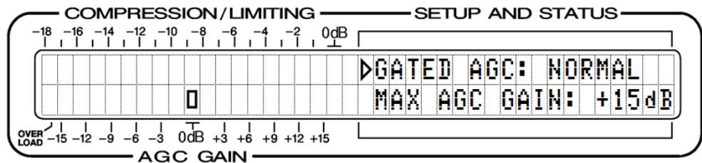
The AGC has a ‘resting’ value at the 0dB point on the AGC GAIN scale. A proper adjustment of Model 261 input gain causes the AGC to hover around the 0dB mark most of the time that the AGC is operating. When the gate closes, AGC gain will slowly return to the 0dB resting point.
