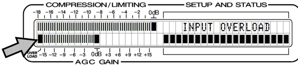
This primary alarm has an *integrated* peak response to program signal overloads, allowing the occasional transient to slip through. However, a secondary indicator, marked OVERLOAD (arrow) has instantaneous peak response. This secondary flasher is held for a sufficient period to make even the briefest overload visible to the operator.
