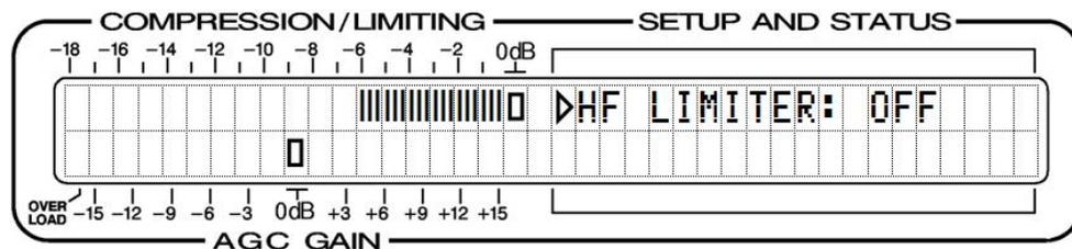
With the ◀ and ▶ select buttons, the HF limiter can be set to protect either the 50 $\mu$ s or 75 $\mu$ s pre-emphasis transmission curves:
