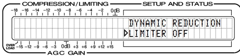
Operating mode choices are made with the ◀ and ▶ select buttons. These are: LIMITER OFF, PEAK LIMIT ONLY and LIMIT AND COMPRESS. The independent high frequency, pre-emphasis-protection limiter is a separate function and is discussed on Page 20.
