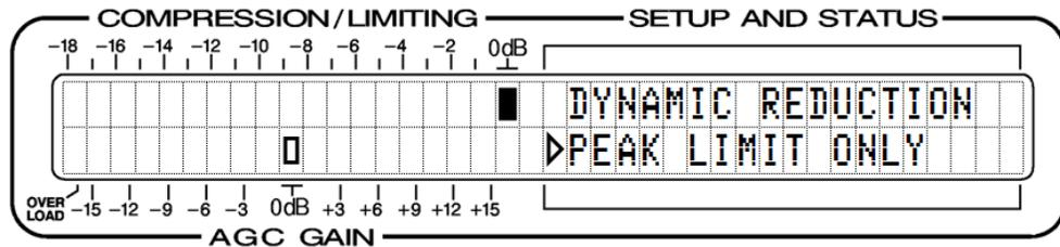
In the limit-only mode, limiter action is not gated. Note the solid block at 0dB on the COMPRESSION/LIMITING scale. Also note that AGC has been enabled in this case, and that the gate is closed.
