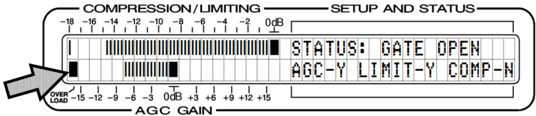
This alarm is located in the lower, left-hand corner of the screen and indicated by the arrow here. This alarm is shared with the input-overload-sensing circuit, which is discussed at the top of Page 14. This alarm has no associated tally output.
