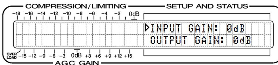
With the ▷ cursor set as shown above, the ◀ and ▶ buttons allow adjustment of the input gain over a  $\pm 15$ dB range in 1dB steps. This setting applies to either the analog or the digital inputs, whichever is selected. *There is no provision for independent gain settings for analog and digital input signals.* If the two input modes are used alternately, then input gain may have to be reset when the selection is changed.
