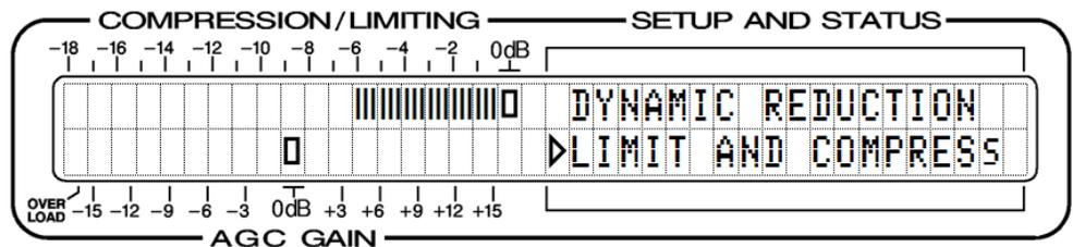
Compression is gated, the same as the AGC, and in the illustration above the gate is closed. Compression will seek its -6dB resting value just as the AGC seeks 0dB.
