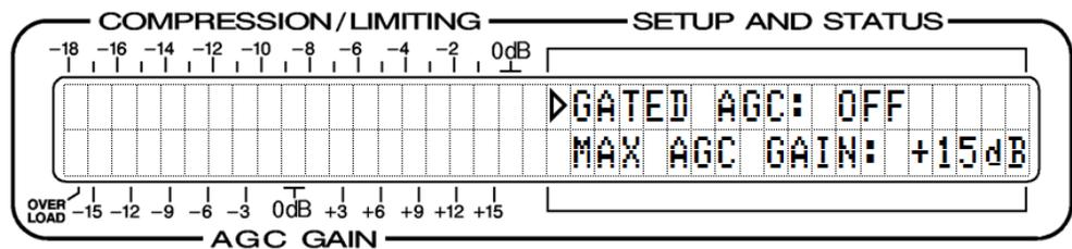
With the ▷ cursor positioned as shown above, ◀ and ▶ may be used to toggle the AGC among its three modes: OFF, NORMAL and FAST.
