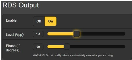
Phase (° degrees): of the RDS subcarrier (relative to stereo pilot phase) should remain at the 90-degree factory preset unless you have a very special reason to change it.
