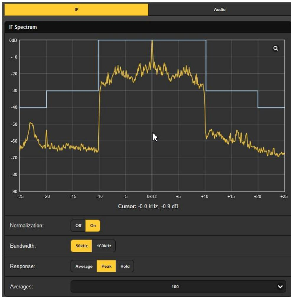
Clicking the magnifying glass in the corner will toggle to a full-screen display, and mousing over the display area brings up a cursor, the white arrow & vertical line shown in the example. The exact frequency and level at that point is noted just below the spectrum.
