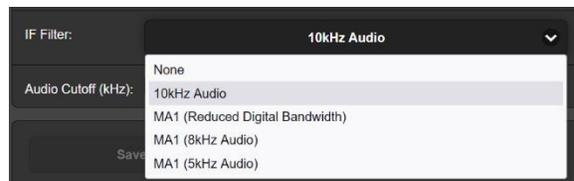
The 10kHz Audio filter may prove the most useful, particularly with off-air listening. Remaining choices are for ‘hybrid mode’ operation, where the AM analog channel is transmitted with one or more HD Radio digital program channels.
