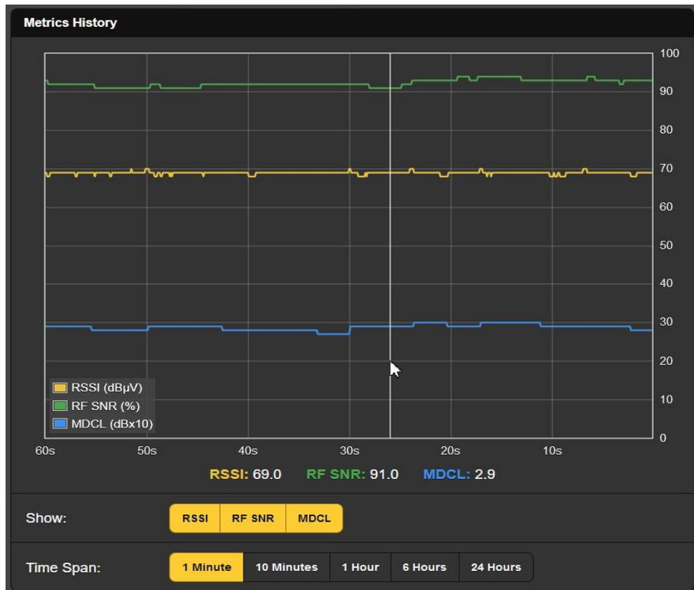
Note the white arrow and line cursor 20-plus seconds-past on the timeline. This cursor will allow you to measure the parameter values anywhere within the displayed timeframe. The nu-
