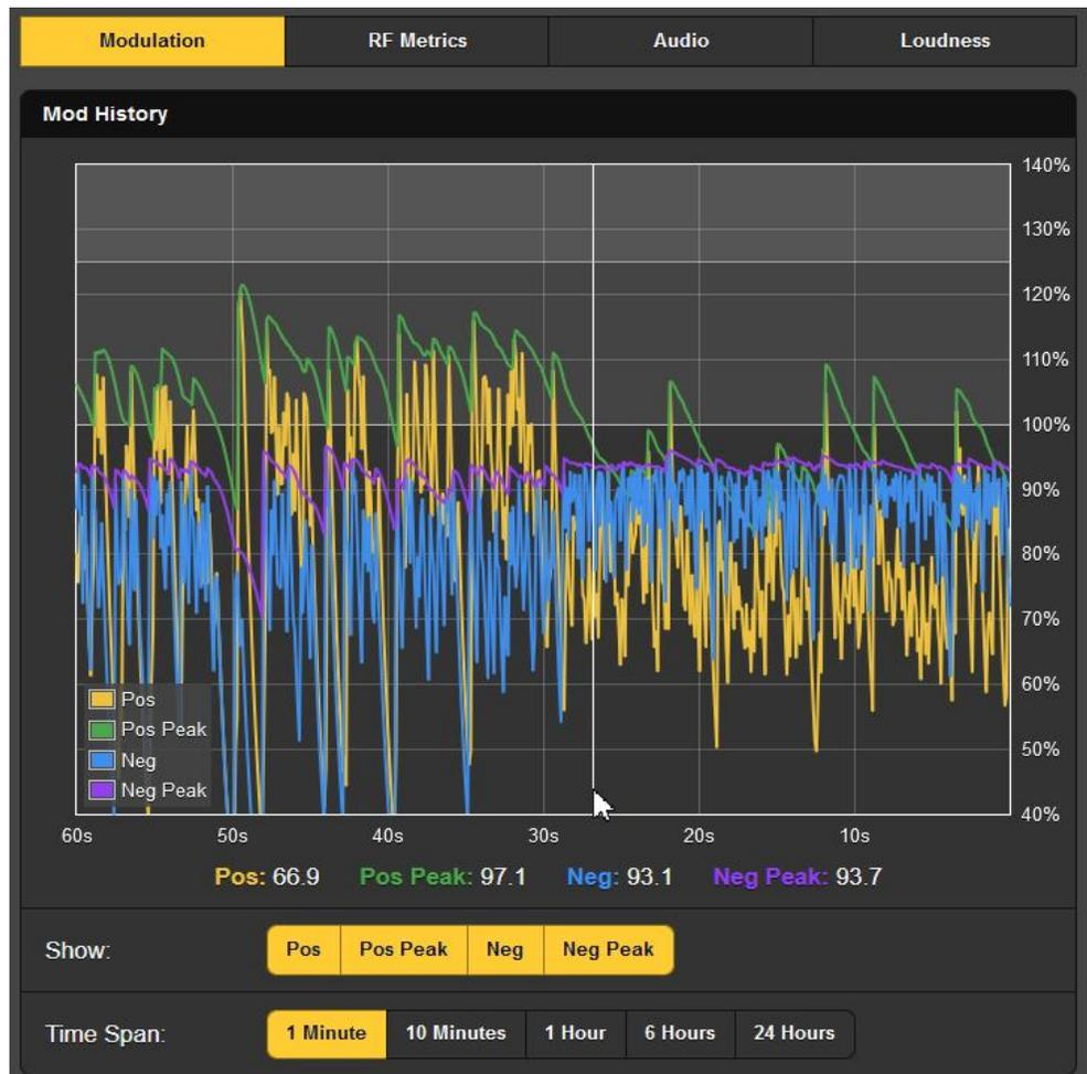
**Modulation** The Modulation screen plots an integrated value of instantaneous positive carrier modulation in yellow (Pos), and a held-peak (Pos Peak) value in green. Ditto for negative modulation, in blue and purple, respectively.
